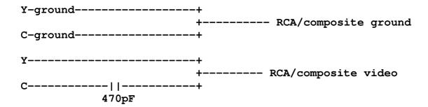
This circuit can be quite easily build inside a the S-video connector case if a physically small size 470 pF (ceramic) capacitor is used. Larger capacitor values will also work, but cause picture to become "softer". The voltage rating of capacitor can be 10V or more.
